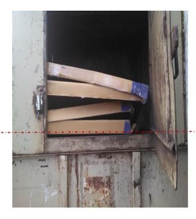
**Problem:** Boxes too large and not completely broken down. Make sure boxes and trash below the red line before compacting.
